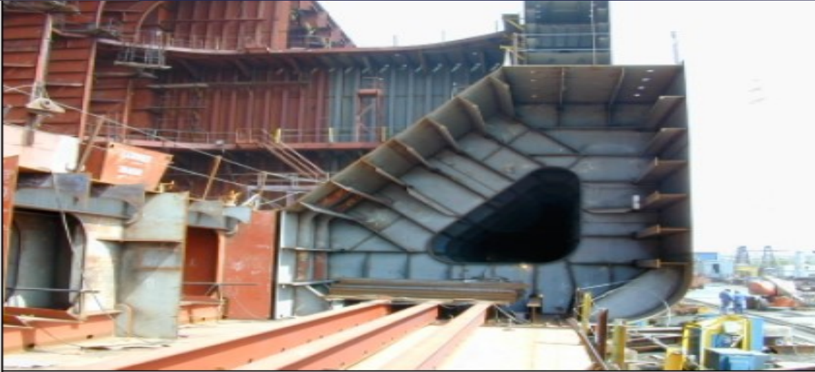
Fig. A5 View of Hopper After Erection, Looking Aft
