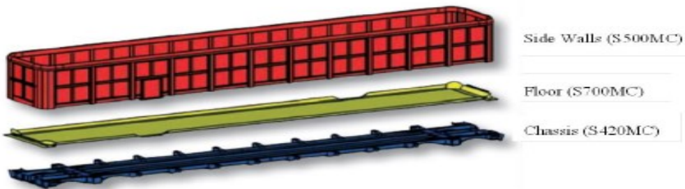
Figure 28 E71-type gondola wagon (ArcelorMittal, 2011)
