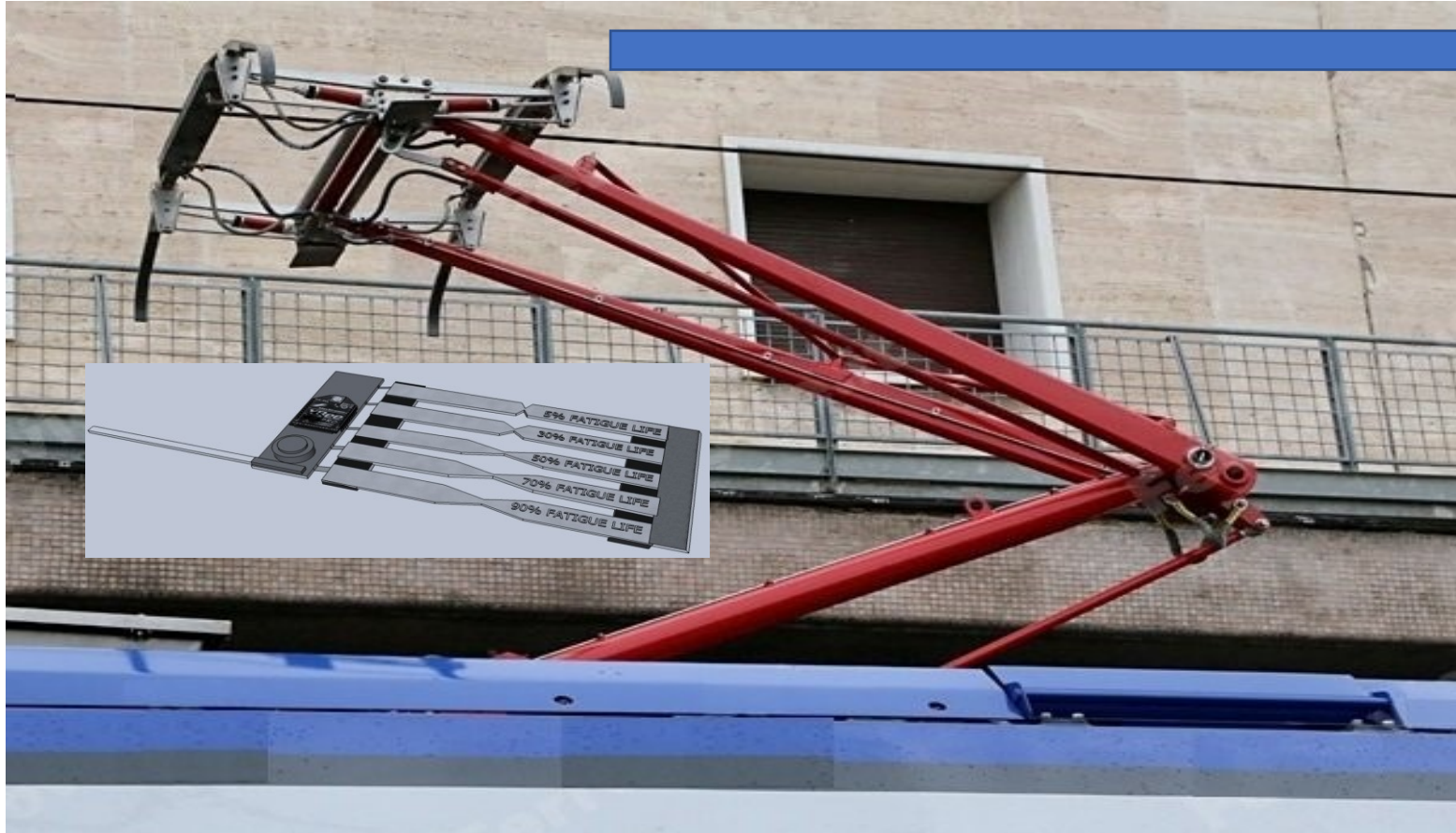
Wireless Enabled SHM-RFID-IoT Smart Fatigue Damage Sensor Network
